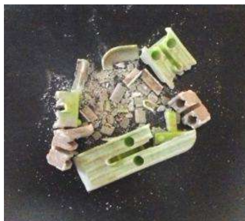
Fig.1. Fragmentation and crumbling of a moulded plastic clothes pin exposed to sun for few months
